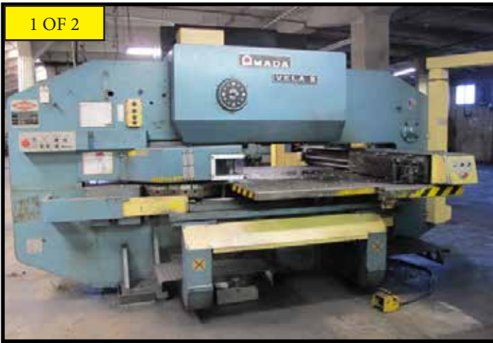
Amada VELA II mdl. VELA II-305050 30-Ton 56-Station CNC Turret Punch Press s/n VII-55363 w/ Amada-Fanuc-V System 6M Controls, 56-Station Turret, Manual Sheet Repositioner, 100" x 50" Ball-Top Table
