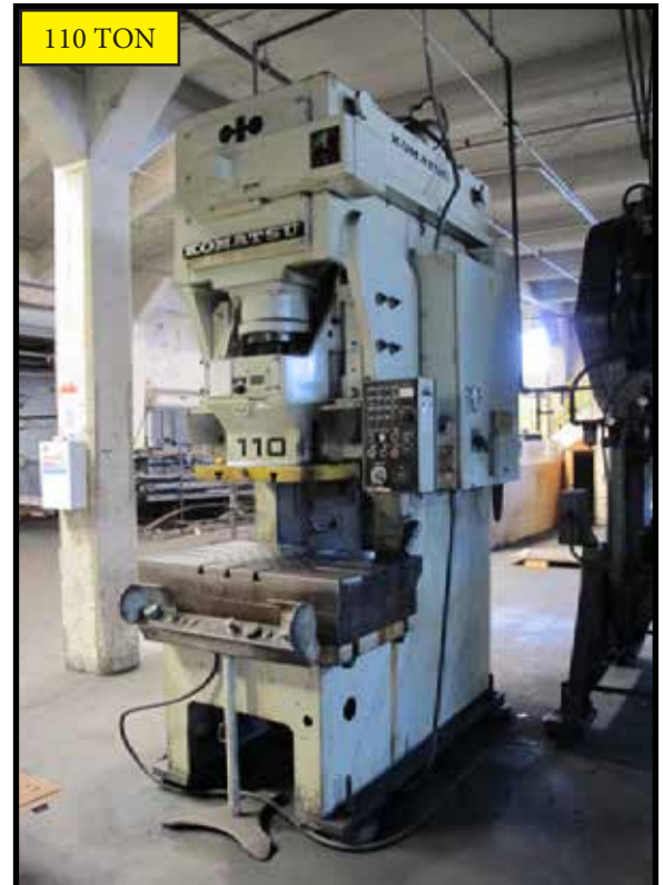
Komatsu OBS110-2 110-Ton Hydraulic Straight Side Press
