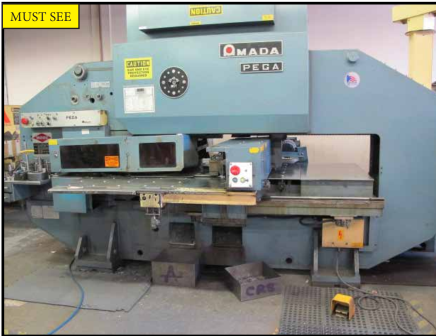
Amada PEGA 304040 30 Ton 40-Station CNC Turret Punch Press w/ Amada-Fanuc-P (System 6M) Controls
