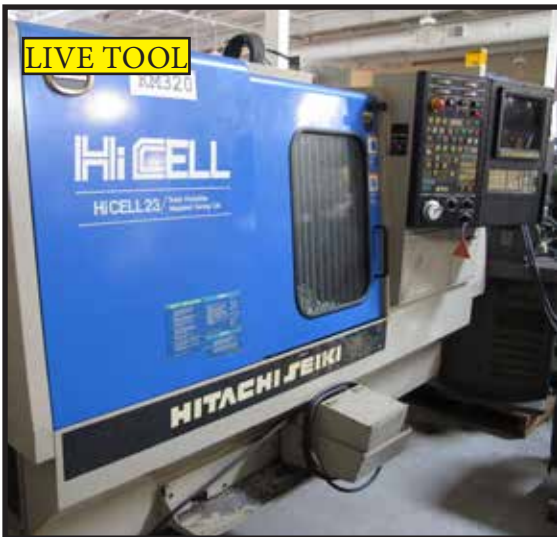
HITACHI SEIKI HI CELL 23, LIVE TOOL CNC TURNING CENTER, WITH C AXIS, Y AXIS, 10 POSITION TURRET, 12 POSTION TOOL CHANGER, SEICOS CONTROL.LNS BAR FEED.
