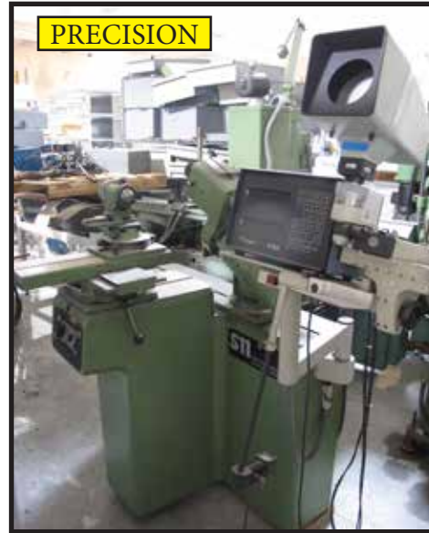
DECKEL S11 UNIVERSAL TOOL AND CUTTER GRINDER WITH OPTO ELECTRONIC MEASURING SYSTEM, DRO AND VARIOUS ATTACHMENTS AND OPTIONS.
