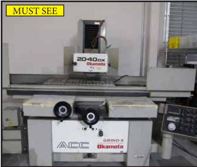
OKAMOTO ACC2040-DX HYD SURFACE GRINDER W/ DIGITAL CONTROLS, 12" X 2" MAXWHEEL SIZE, S/N 70131.
