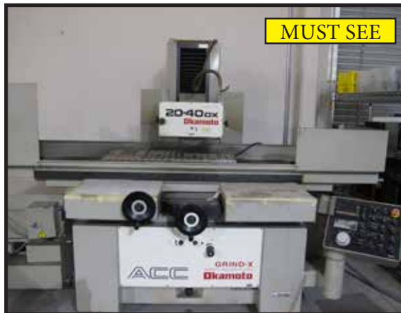
OKAMOTO ACC2040-DX HYD SURFACE GRINDER W/ DIGITAL CONTROLS, 12" X 2" MAXWHEEL SIZE, S/N 70131.
