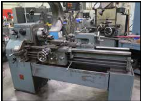
LeBlond Regal Servo Shift 15 1/2" x 45" Lathe s/n 6C289 w/ Sony DRO, 45-1800 RPM, Inch Threading, Tailstock, Steady Rest, KDK Tool Post, 10" 6-Jaw Chuck
