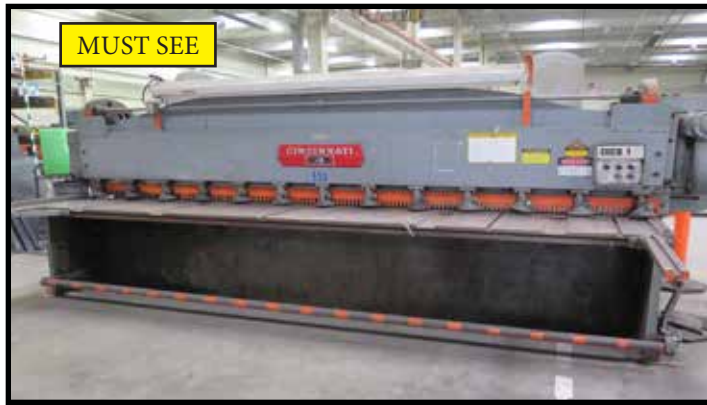
Cincinnati mdl. 1812 18GA x 12' Deep Throat Power Shear s/n 35394 w/ Controlled Back Gaging, 18" Throat, 130" Squaring Arm
