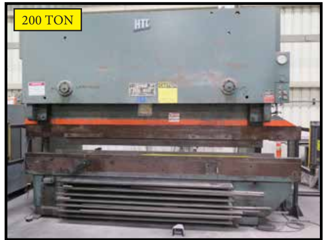
HTC 200G 200 Ton x 13' Hydraulic Press Brake s/n 473668 w/ Power Back Gaging, 8 1/2" Throat, 125.5" Between Uprights, ISB Light Curtain, Front Support Arms
