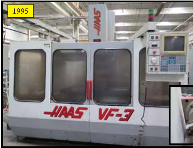
1995 Haas VF-3 CNC Vertical Machining Center s/n 4700 w/ Haas Controls, 20-Station ATC, CAT-40 Taper Spindle, 7500 RPM, Rigid Tapping, Programmable Coolant Nozzle, Chip Auger
