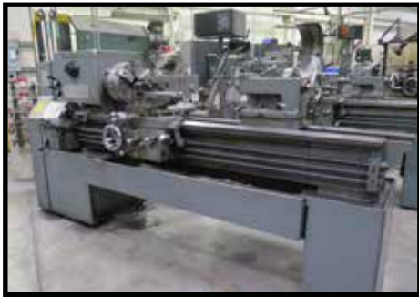
LeBlond Regal Servo Shift 19" x 58" Lathe s/n 12E-524 w/ Sony DRO, 3" Bore Thru Spindle, 40-1600 RPM, Inch/mm Threading, Tailstock, KDK Tool Post, 16" 4-Jaw Chuck
