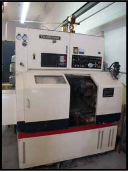
TAKISAWA MODEL TC-2 CNC LATHE, WITH 8" CHUCK, 8 STATION TURRET, 4000 RPM, TAIL STOCK, S/N THRDR4431
