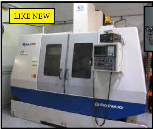
1999 DAEWOO MYNX 500 CNC VMC WITH FANUC 21-M AND MEMERY ENHANCER, 24 ATC, BOX WAYS, CERAMIC BEARINGS, 8000 RPM, 40.2" Z 20.1" X 22.6" (XYZ), S/N AV5E0076.
