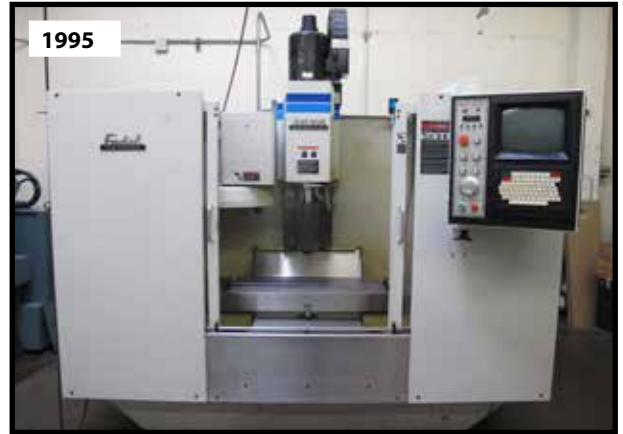
1995 1995 FADAL MODEL VMC-3016 CNC VMC, CT-40 TAPER, 20 ATC, CNC88HS CONTROL, S/N 9502107.
