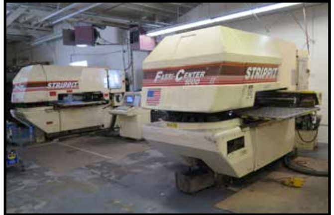
Strippit Fabri-Center 1000 II mdl. FC1000 XP II 22.5-Metric Ton x 20-Station CNC Turret Punch Press s/n 079122094 w/ Macintosh Computer Controls,
