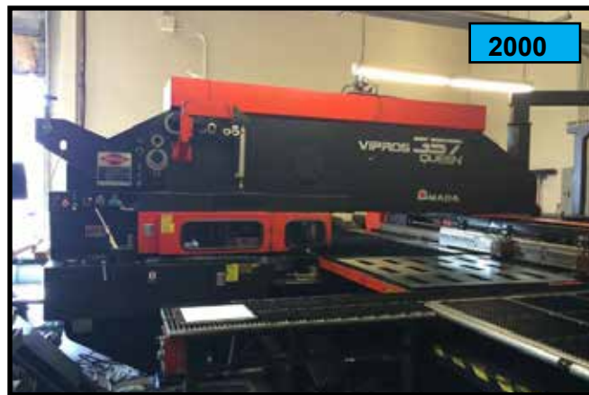
2000 Amada Vipros QUEEN 33-Ton 58-Station CNC Turret Punch Press s/n AVU57187 w/ Fanuc 18-PC Controls, (2) Auto Indexing Stations, 50" x 72" Travels, 50" x 144" Max Sheet Size,
