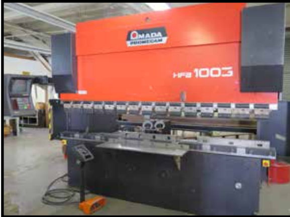
1997 Amada Promecam HFB1003 1000kN x 122" CNC Press Brake s/n HFBO100-30-R970707 w/ Amada Operateur Controls,
