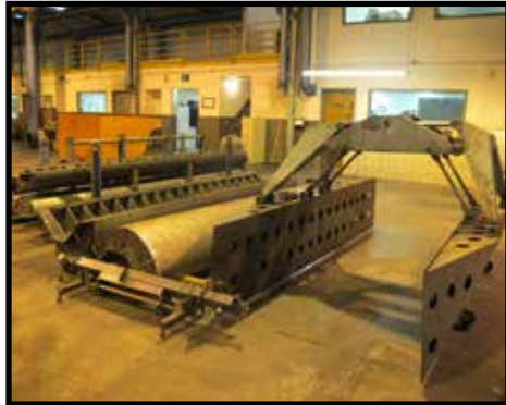
SPIRO NO 1 FLAT OVAL STRETCHER WITH 14" TO 24" X 12FT MANDRELS IN INCREMENTS, AND 30" X 12FT MANDREL.
