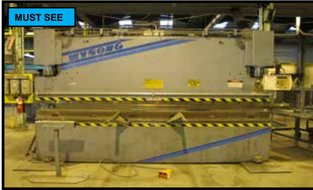
WYSONG MTH140-144, 12FT X 140 TON HYD CNC PRESS BRAKE, WITH AUTOGAGE 99 CNC BACK GAGE, S/N MT5-124
