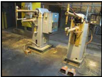
ACME SPOT WELDER W/CONTROLS 75 KVA CAP
