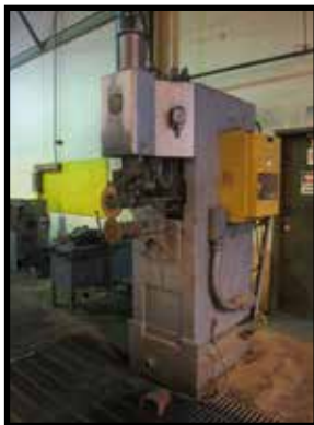
BANNER 150 KVA SEAM WELDER WITH ENTRON CONTROLS.
