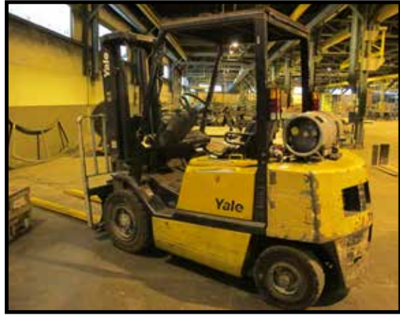
YALE 5000 LB LPG FORKLIFT WITH PNEUMATIC TIRES, SIDE SHIFT, APPROX 1600 HOURS, 2 STAGE.
