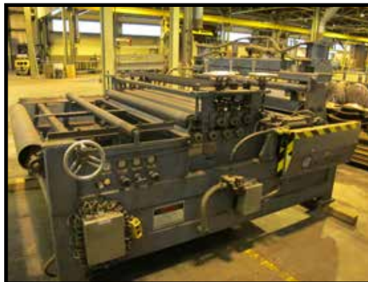
IOWA PRECISION CUT TO LENGTH LINE, MODEL CTL-616, 60" X 16GA CAP, WITH UMC 4FT UNCOILER, CRADLE CAR, AND CONTROLLER, S/N 58509.
