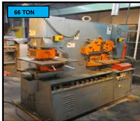
MARVEL SPARTAN IW66D, 66 TON HYDRAULIC IRON ORKER.
