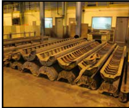
SPIRO NO 1 FLAT OVAL STRETCHER WITH 14" TO 24" X 12FT MANDRELS IN INCREMENTS, AND 30" X 12FT MANDREL.
