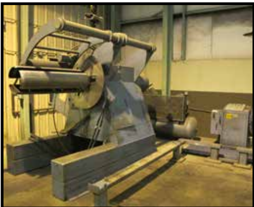
IOWA PRECISION CUT TO LENGTH LINE, MODEL CTL-616, 60" X 16GA CAP, WITH UMC 4FT UNCOILER, CRADLE CAR, AND CONTROLLER, S/N 58509.
