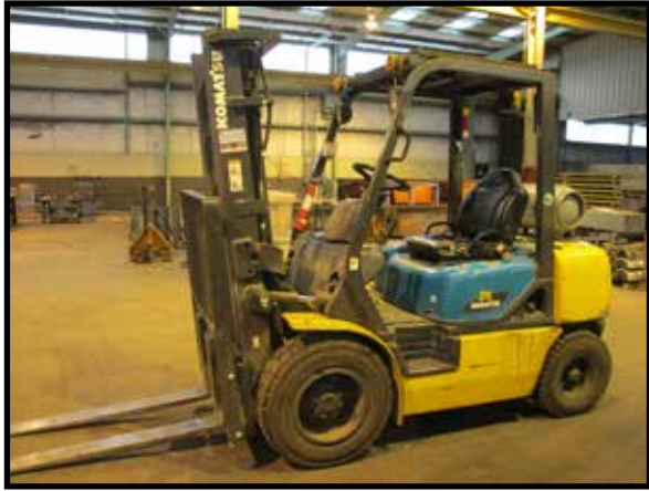
KOMATSU 5000 LB LPG FORKLIFT WITH PNEUMATIC TIRES SIDE SHIFT, APPROX 2800 HOURS.
