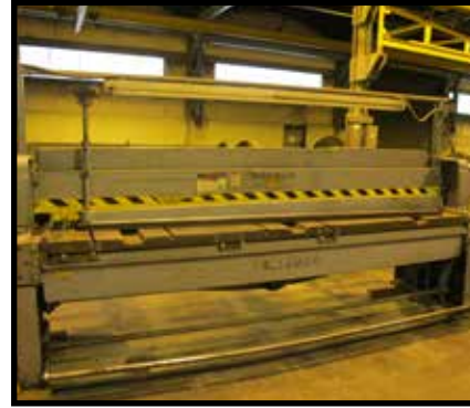
WYSONG 1010, 10FT X 10GA MECHANICAL POWER SHEAR.
