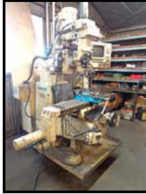
MILLTRONICS "PARTNER" MDL.4 SERIES F CNC VERTICAL MILL S/N 3401 W/ CENTURION I CONTROLS, 5HP MOTOR, 50-3750 RPM, KURT POWER DRAW BAR, 40-TAPER SPINDLE, POWER KNEE FEED.
