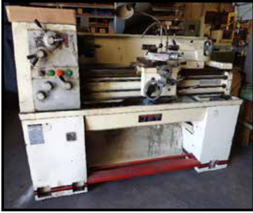
JET GH-1340A 13" X 40" GEARED HEAD GAP BED LATHE S/N 805W360 W/ TAILSTOCK, STEADY REST.
