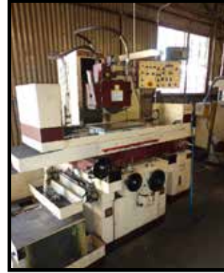
FALCON CHEVALIER FSG-1020AD 10" X 20" AUTOMATIC HYDRAULIC SURFACE GRINDER W/ SONY DRO, HYDRAULIC WHEEL DRESSER.
