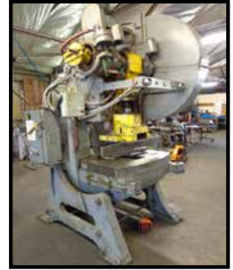
V & O PRESS CO NO.5 1/2 55-TON OBI STAMPING PRESS S/N 555-42 W/ PNEUMATIC CLUTCH.
