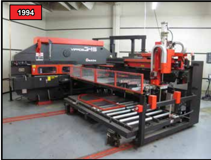
1994 1994 AMADA VIPROS 345, 33 TON CNC TURRET PUNCH, WITH FANUC O4PC CONTROL, 58 STATION, 2 AUTO INDEX, AND AMADA MP1212NF LOAD SYSTEM, S/N AVP45027.
