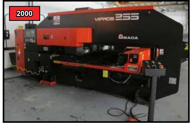
2000 2000 AMADA VIPROS 255, 22 TON CNC TURRET PUNCH, WITH FANUC 18-P CONTROL, BRUSH TABLE, 3 AUTO INDEX, THICK TURRET, 31 STATION, S/N AVP55285.
