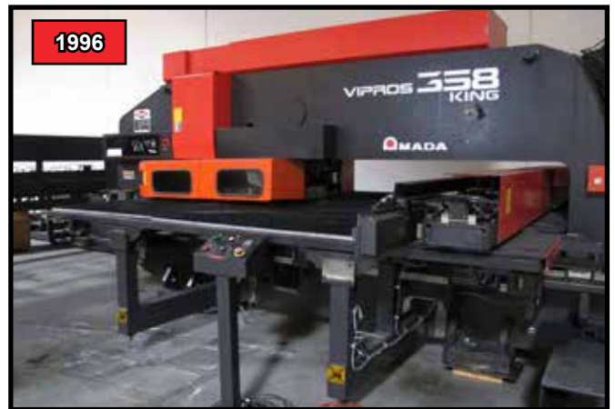
1996 1996 AMADA VIPROS 358 KING, 33 TON CNC TURRET PUNCH, WITH AMADA O4PC CONTROL, 58 STATION, BRUSH TABLE, 2 AUTO INDEX, S/N 35820284.
