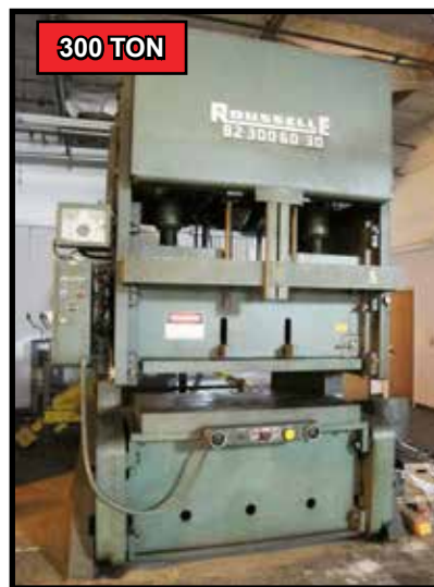
ROUSSELLE B2-300-60-30, 300 TON GAP FRAME PUNCH PRESS, 35 SPM, 4" STROKE, 18" SHUT HEIGHT, 60" X 30" TABLE, S/N 23102.
