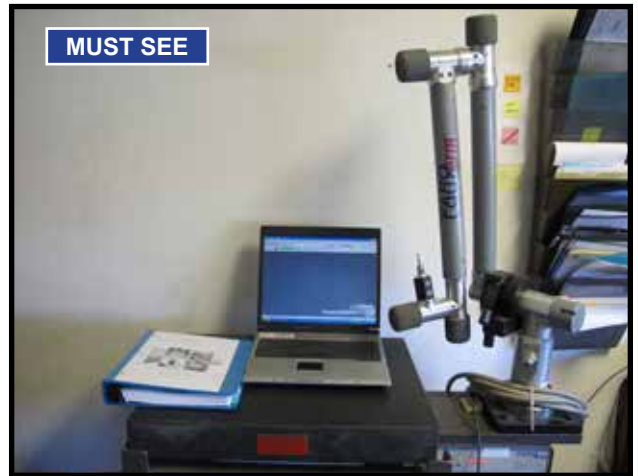
FARO ARM SILVER CMM WITH 60" CUBE CAPACITY, 18" X 24" GRANITE TABLE AND WITH ALL NEW UPDATED SOFTWARE AND COMPUTER, S/N S08029600449.
