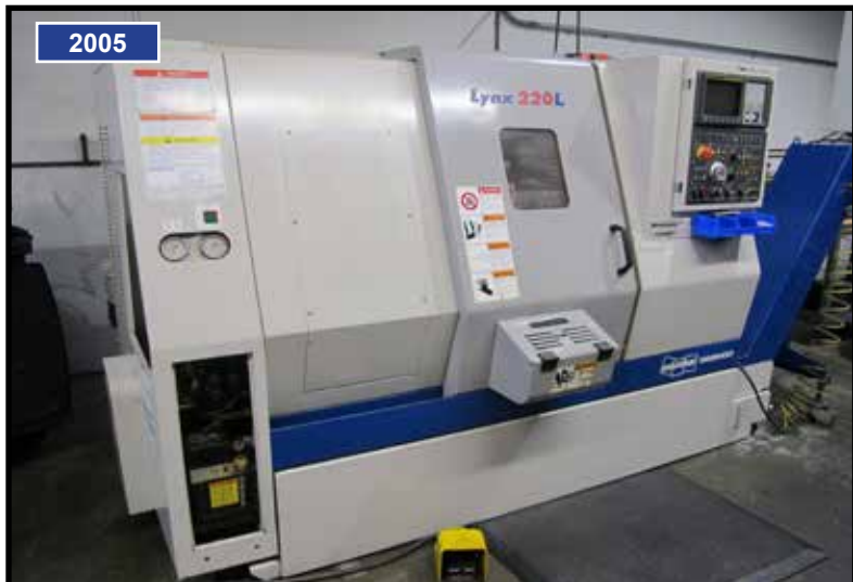
2005 DOOSAN-DAEWOO LYNX 220 LC CNC TURNING CENTER, WITH FANUC CONTROL, CHIP CONVEYOR, TAIL STOCK, 12 POSITION TURRET, PARTS CATCHER, 8" CHUCK, S/N L2200704.
