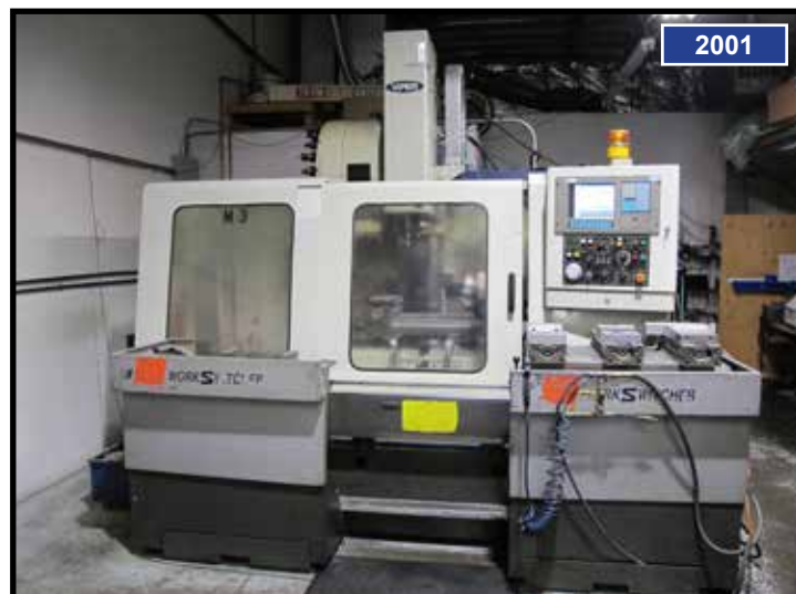
2001 MIGHTY VIPER VMC-950-AG, 40" X 20" X 20" (XYZ) CNC VMC, CT-40, 21 ATC, WITH MITUSBIHI MAGIG 64 CONTROL, 8000 RPM, 2 SPEED GEAR HEAD, RIGID TAPPING, FULL 4TH AXIS READY AND TROYKI 4TH AXIS ROTARY TABLE, S/N 003196.
