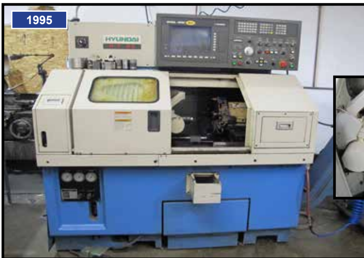
HYUNDAI HIT-HS TURNING CENTER, W/HITROL-840 C CONTROL, CHIP CONVEYOR, 15C COLLET NOSE, PARTS CATCHER
