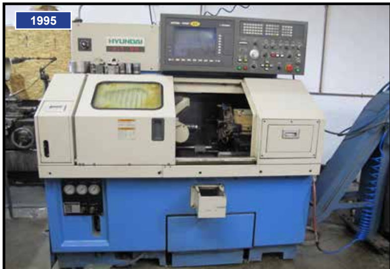
1995 HYUNDAI HIT 8S CNC TURNING CENTER WITH HITROL 840C EZ CONTROL, TURBO CHIP CONVEYOR, 8 STATION TURRET, 15C COLLET NOSE, PARTS CATCHER, S/N 5083.
