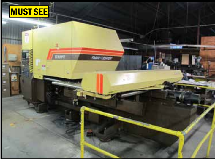
1992 STRIPPIT FC1000 III, 33 TON CNC TURRET PUNCH W/ FANUC 6M CONTROL, AUTO INDEX
