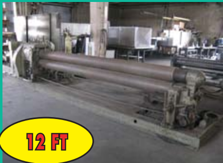
WEBB MODEL 6L, 12FT x 3/16" INITIAL PINCH PLATE ROLLS
